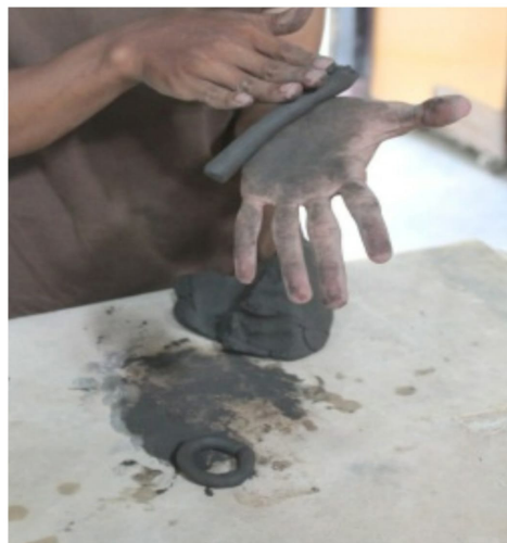
Photo 1 Clay plasticity test on the LSM and MMYA mixture.
