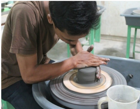
Photo 5 The process of making ceramics using the throwing technique.
