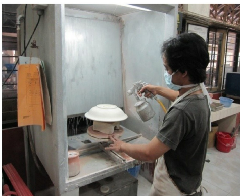
Photo 8 The glazing process for stoneware ceramics.
