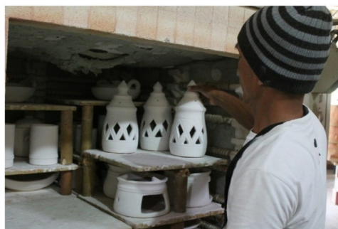
Photo 9 The firing process for glazed ceramics.
