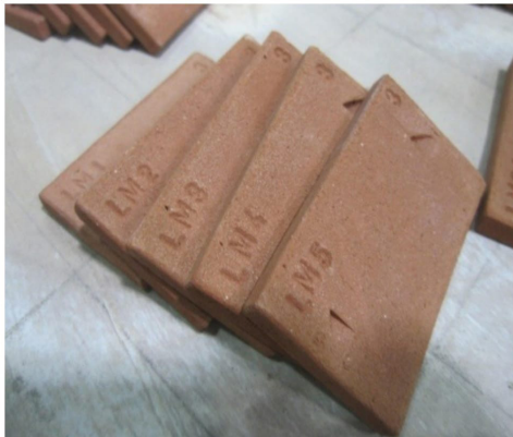
Photo 3 Firing shrinking clay test result of LSM and MMYA.
