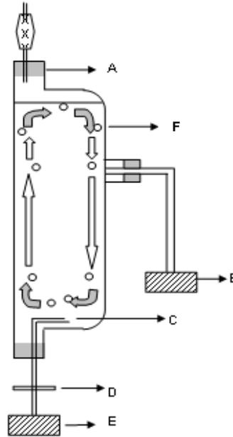
**Figure 1:** Schematic diagram of a tubular air-lift fermenter: A – gas exit (vent), B – sampling port, C – sparger, D – air filter, E – air pump, F – turbulent/direction of medium flow. The arrows indicate the flow of the medium.
