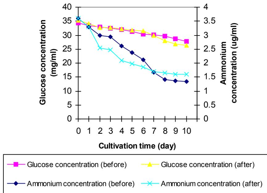
**Figure 4:** Time course of glucose and ammonium concentrations before and after optimization in a tubular air-lift fermenter.
