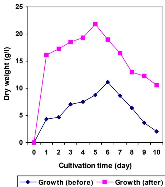
**Figure 5:** Time course of fungal growth of *H. grisea* before and after optimization in a tubular air-lift fermenter.
