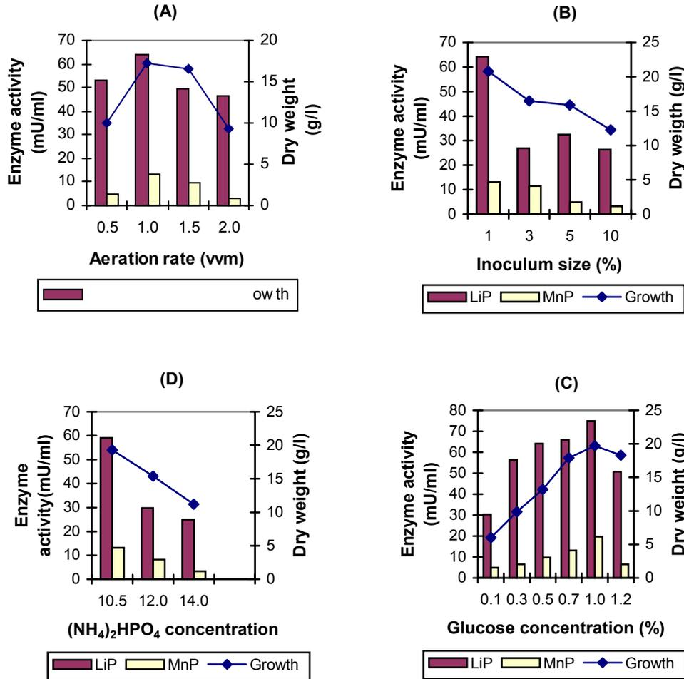
**Figure 2:** Effects of (A) aeration rate, (B) inoculum size, and (C)  $(\text{NH}_4)_2\text{HPO}_4$  and (D) glucose concentrations, on the production of LiP and MnP by *H. grisea* in a tubular air-lift fermenter system.
