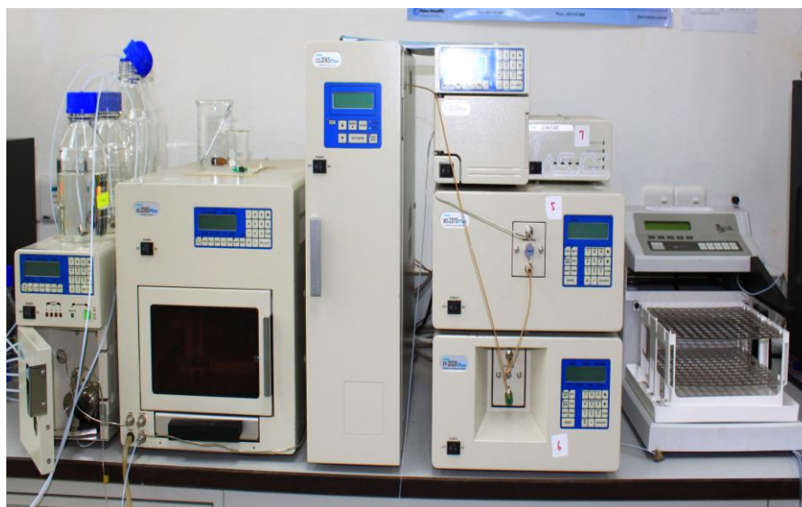
Figure 4: The main components of a modern HPLC system.
