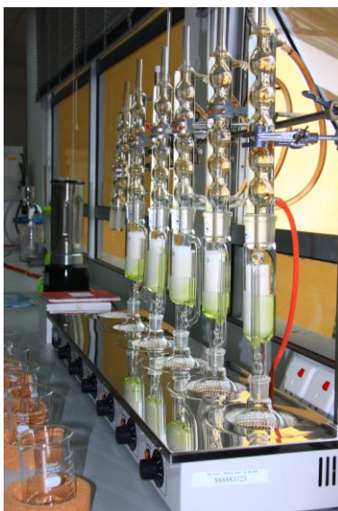
Figure 2: Soxhlet used for conventional solvent extraction which is still relevant today.
