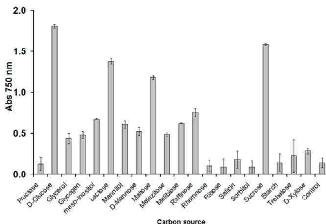
**Figure 3:** The effect of various carbon sources as electron donors for molybdenum reduction to molybdenum blue by *Bacillus* sp. strain Neni-10. The error bars indicate mean  $\pm$  standard deviation of three replicates.
