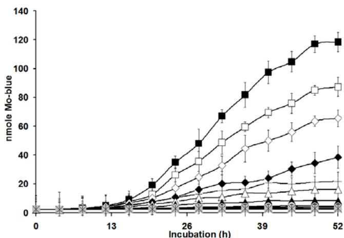
**Figure 6:** A time profile of molybdenum blue production at sodium molybdate concentrations of 0 (\*), 5 (×), 10 (+), 15 (□), 20 (■), 25 (◇), 30 (◆), 35 (△), 40 (▲), 50 (○), 60 (●) and 70 mM (\*). The absorbance values measured at 750 nm were converted to Mo-blue concentration measured as nmole Mo-blue. The error bars indicate mean ± standard deviation of three replicates.
