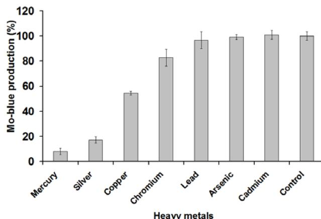
**Figure 7:** The effect of heavy metals on Mo-blue production by *Bacillus* sp. strain Neni-10. The error bars indicate mean  $\pm$  standard deviation of three replicates.
