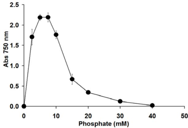
**Figure 4:** The effect of phosphate concentrations on molybdenum blue production. The error bars indicate mean  $\pm$  standard deviation of three replicates.
