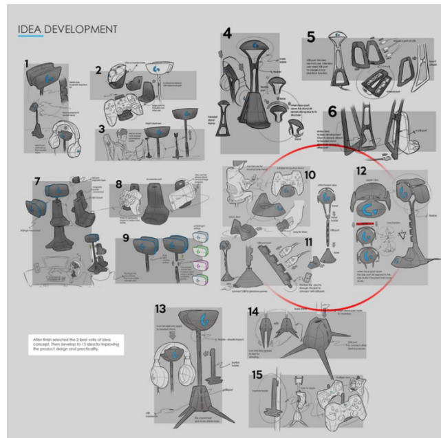
Figure 8 Example of additive innovation of Logitech headset’s stand by student participants. Source: Credit image, Ahmad Aiman Anuar (50595, UniSZA).
